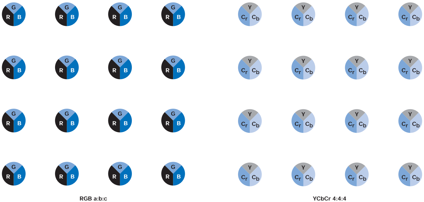
Figure 3. Illustration of RGB a:b:c and YCbCr 4:4:4 Formats.
